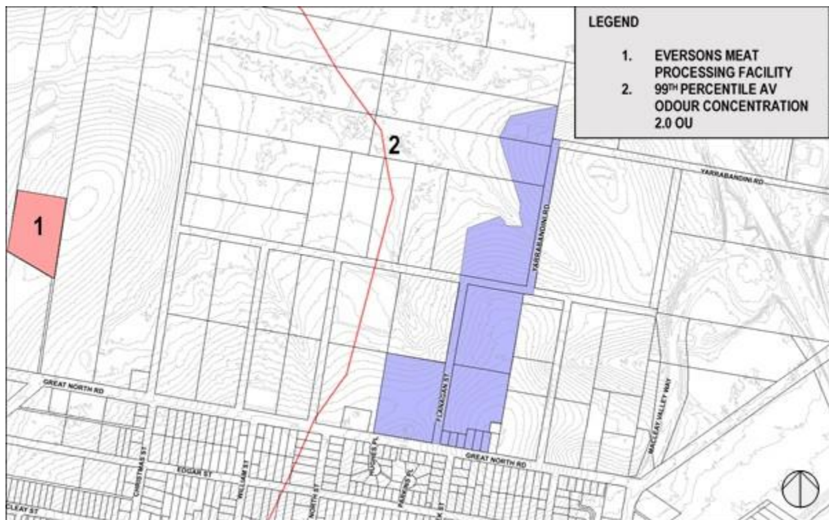
Map 9. Everson Meat Processing Facility Frederickton – 99 th Percentile (1 Second) Average Odour Concentration on the Proposed Re-Zoning Areas (Criterion: 2.0 OU)
